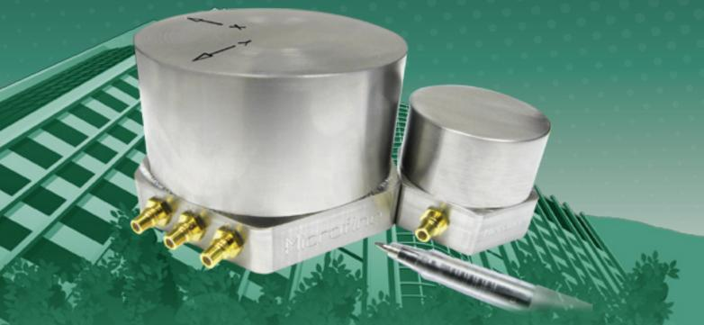
Model SIA1 is an ultra-high sensitivity seismic / infrasonic accelerometer. It incorporates MMT's unique design and PZN-PT single crystal technology and has an extremely wide dynamic range of <1x10<sup>-5</sup> g to 20 g. It is available in both 1-D and 3-D designs. Other performance characteristics are provided in the table below.
